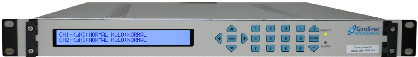
Option 34-7 Front panel display with RS485/422 and Ethernet remote control
