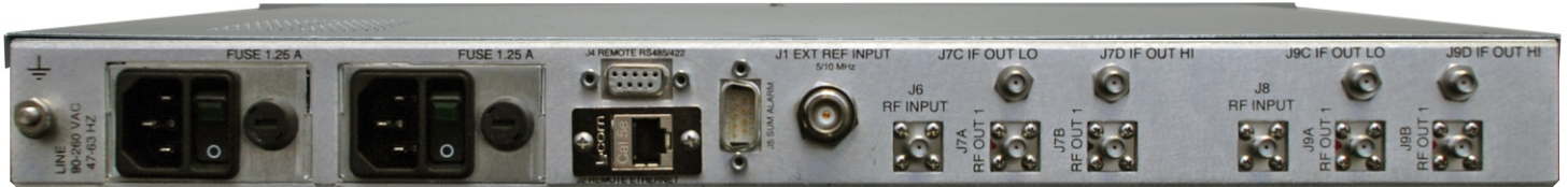
Typical rear panel view - Shown with options 34-3, 5, 6 and 7
